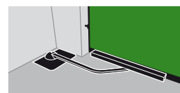
Below-ground motor positioned to the side (when space is an issue)
